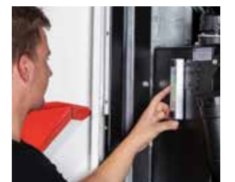
Easy checking of oil levels through windows
