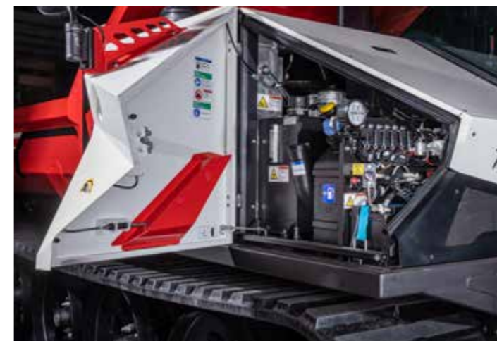
Easy checking of oil levels through windows
